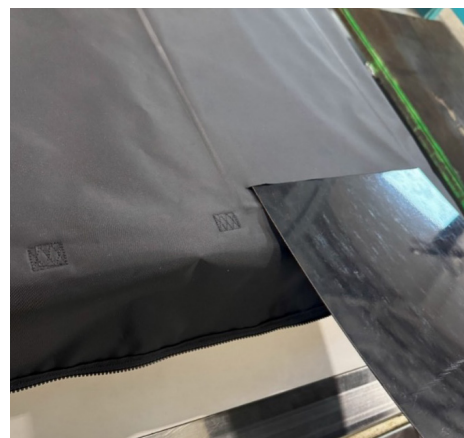
9. Remove the old bottom. Install the plastic panel into the sleeve on the new cover bottom.
