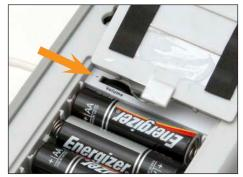
2 Adjust the volume control in the battery compartment, close the cover, and tighten the screw
