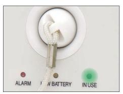
Confirm that the green "IN USE" light is flashing.
