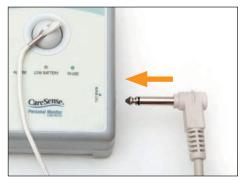
6 CONNECTING TO NURSE CALL: Plug a Nurse Call Connection Cable into the "NURSE CALL" socket on the monitor, connect the opposite end of cable into Nurse Call Station (an adaptor may be required) and test.
