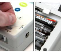
Remove the plastic film from face of the monitor, and install batteries.
