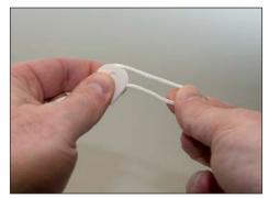
Adjust the string to a length that will pull out the magnetic dome to activate the alarm if the patient attempts an exit.
