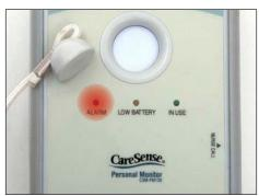
TEST THE ALARM: Remove the magnetic dome from the socket. The alarm will sound, and the red "ALARM" light will flash.
