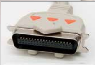
The Centronics connectors on the Curbell breakaway cable have no pins to break.
