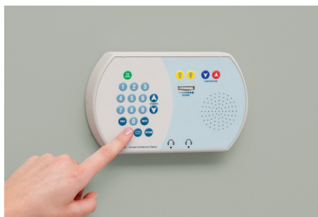
The Remote Entertainment Station provides easy access to the same TV features as a pillow speaker.
