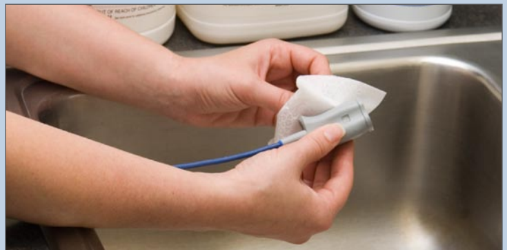
SoftTip probes can be turned inside out for easy and thorough cleaning.
